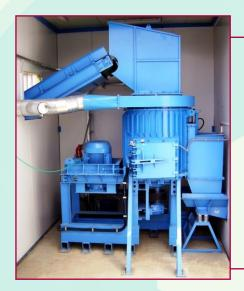
According to the range of waste uses a different engine power and diameter of the working cylinder. Shredding is not continuous. As for the following technology, the output can be sorted simply. A working chain and a carrier conveyer are the material to be consumed. If the resulting explosive dust is inerting needed workspace of the shredder. The shredder should be integrated into the system, whose design and supply of individual components ODES s.r.o. provide.
